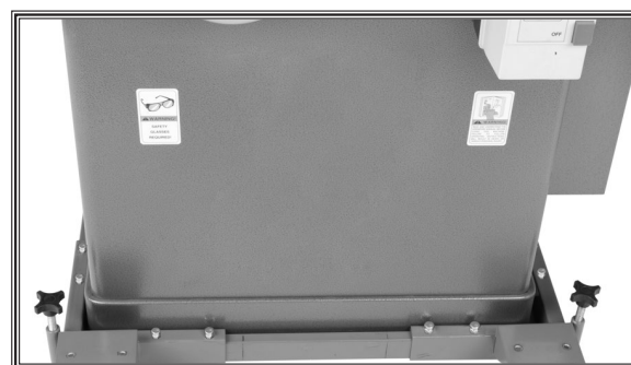
Figure 21. Corner bracket-rail assembly placed under front of machine.
