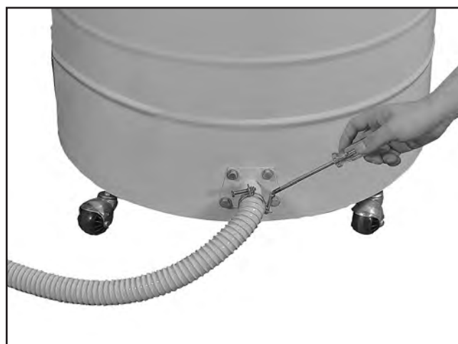
Figure 31. Connecting the vacuum hose.
