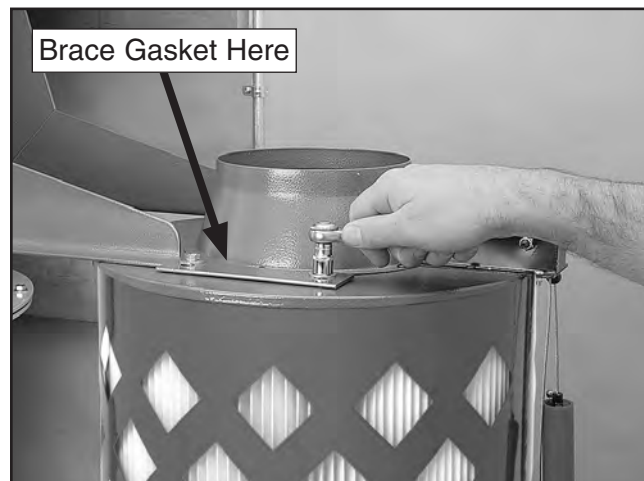
Figure 19. Mounting filters to the braces.
