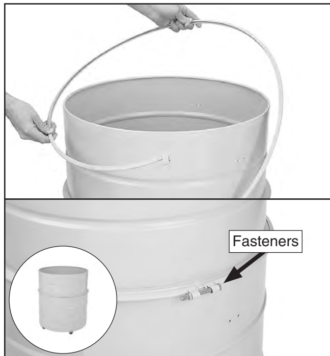
Figure 25. Installing metal clamp around collection drum.
