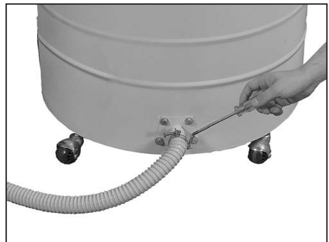
Figure 35. Connecting the vacuum hose.
