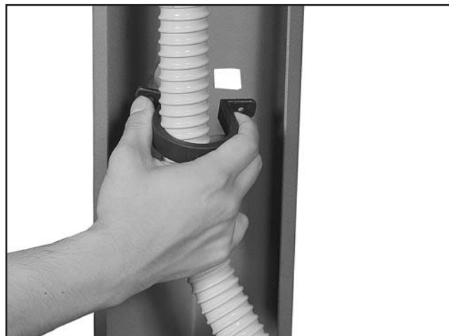
Figure 36. Securing vacuum hose to stand legs.
