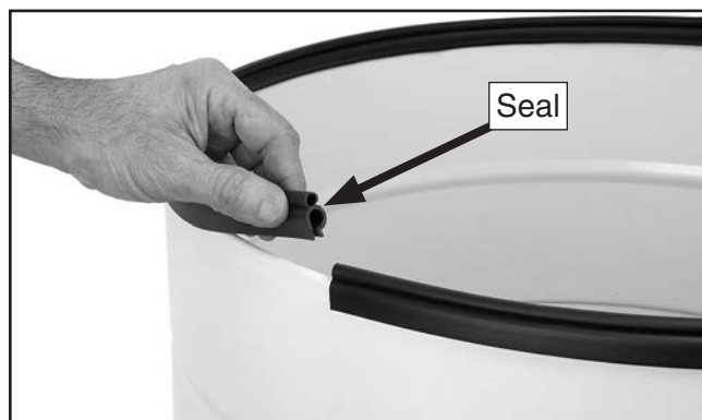
Figure 31. Installing drum lid seal.
