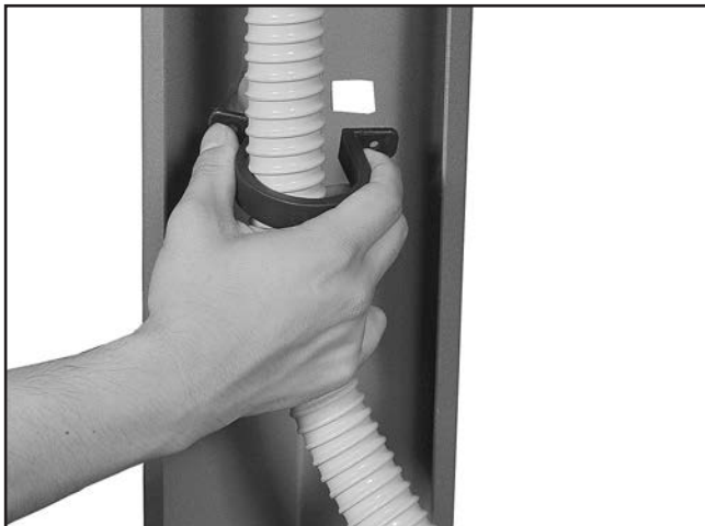
Figure 37. Securing the vacuum hose to the stand legs.
