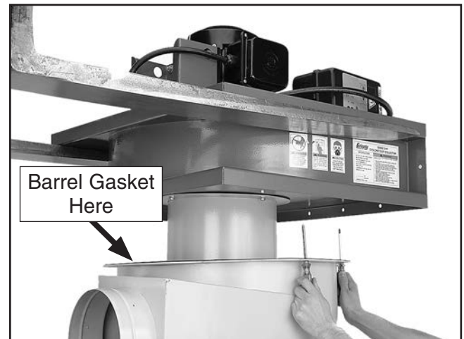
Figure 13. Aligning mounting holes.
