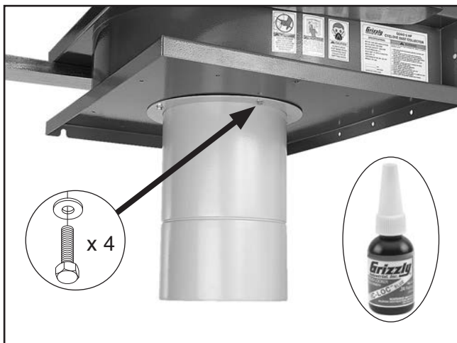
Figure 17. Intake cylinder attached to the bottom of motor/blower housing.
