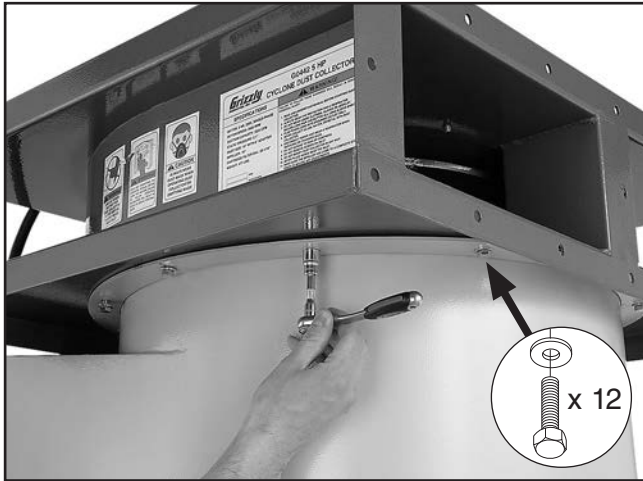
Figure 20. Securing blower on intake barrel.
