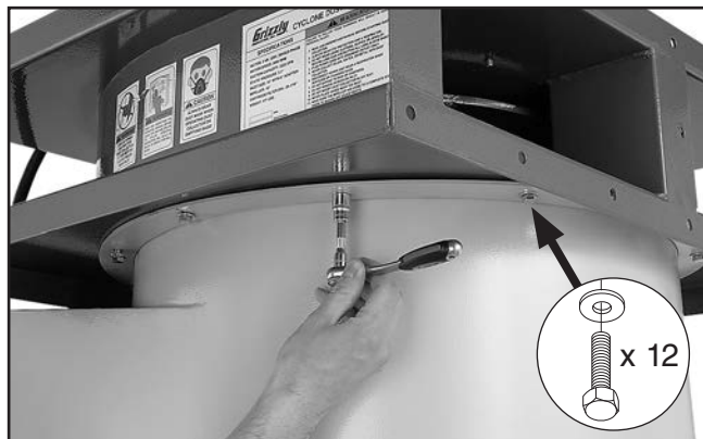
Figure 15. Securing blower on intake barrel.
