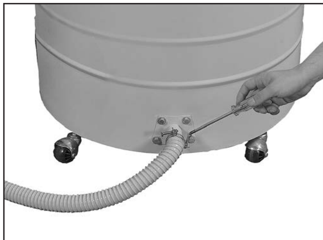
Figure 34. Connecting vacuum hose.
