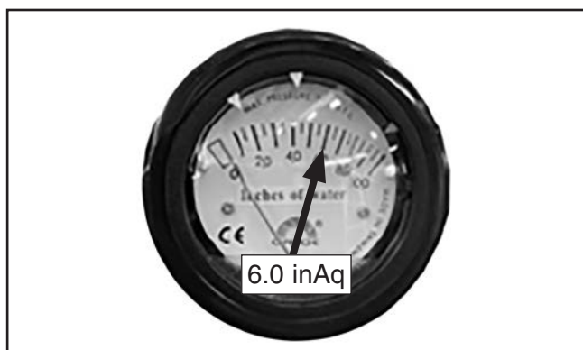
Figure 3. Location of 6 inAq on pressure gauge.
