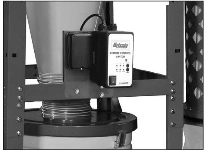
Figure 38. Switch mounted to stand.
