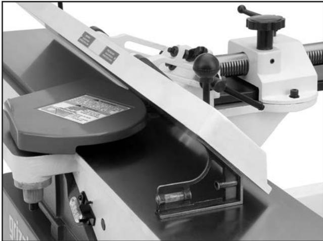
**Figure 72.** Adjusting fence 45° inward.
