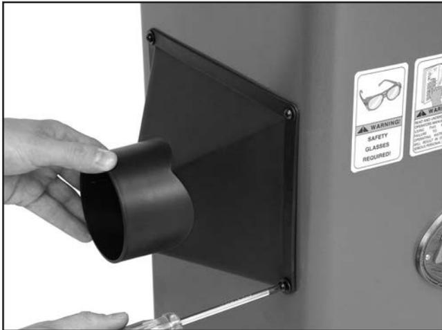
**Figure 25.** Dust port installation.
