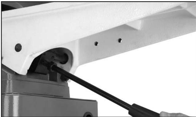
**Figure 29.** Installing infeed table lever.
