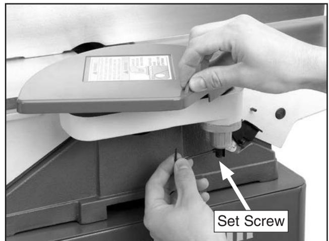
**Figure 24.** Re-installing set screw.
