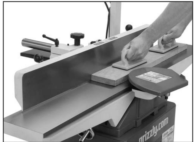
**Figure 43.** Typical surface planing operation.
