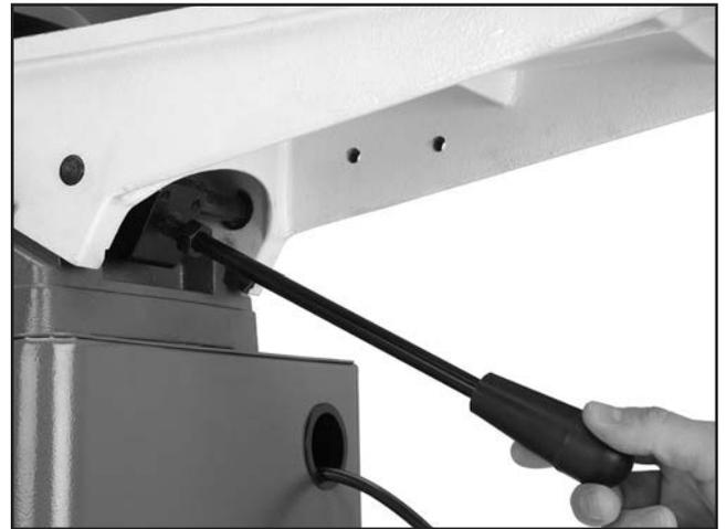
**Figure 39.** Adjusting infeed table height.
