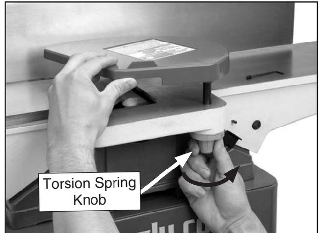
**Figure 23.** Setting torsion spring knob.
