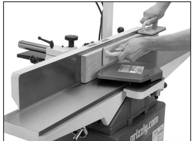
**Figure 45.** Typical edge jointing operation.
