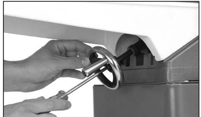
**Figure 28.** Securing the handwheel.
