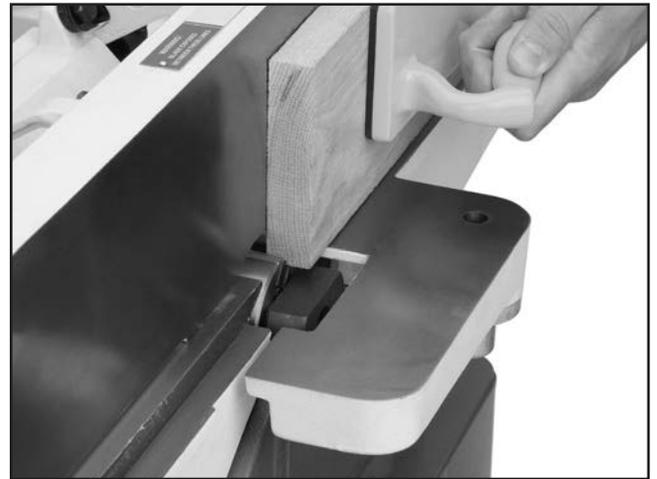
**Figure 49.** Typical rabbet cutting operation.
