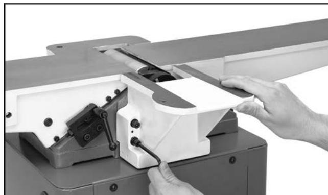
**Figure 18.** Assembled carriage mounting bracket.
