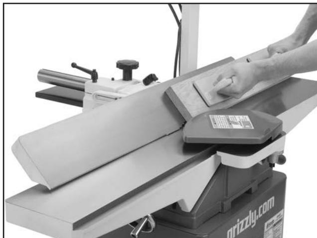
**Figure 47.** Typical bevel cutting operation.
