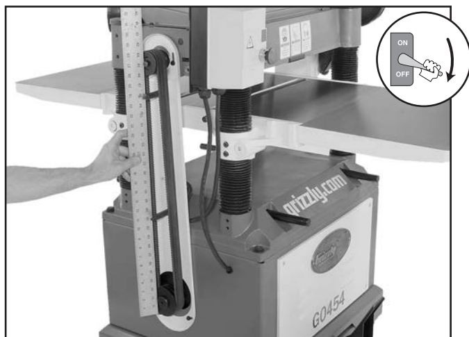
Figure 34. Checking pulley alignment.
