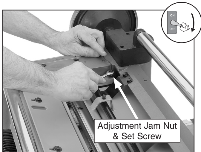
Figure 40. Example of adjusting the pressure bar height.
