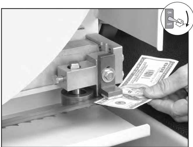
Figure 18. Dollar bill between upper guide block and blade.
