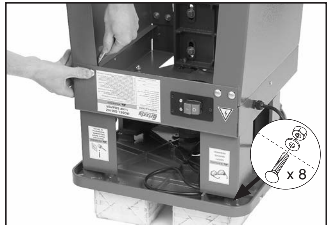
Figure 11. Example of attaching stand to shaper unit.
