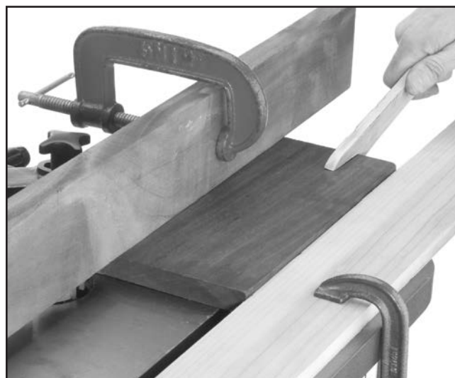
Figure 25. Safety boards and push stick in use.
