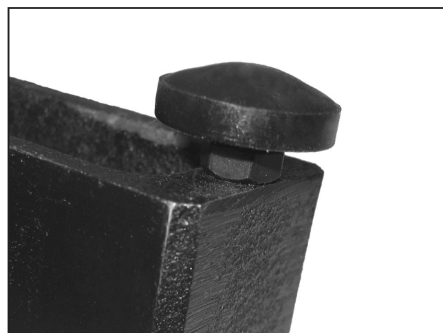
Figure 24. Installed rail pad.
