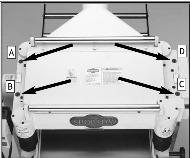
Figure 27. Roller spring tension adjustment screws.
