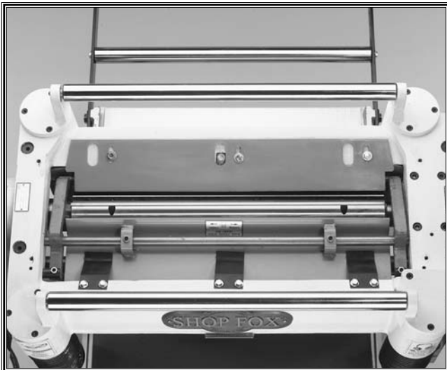
Figure 15. Cover removed from planer.
