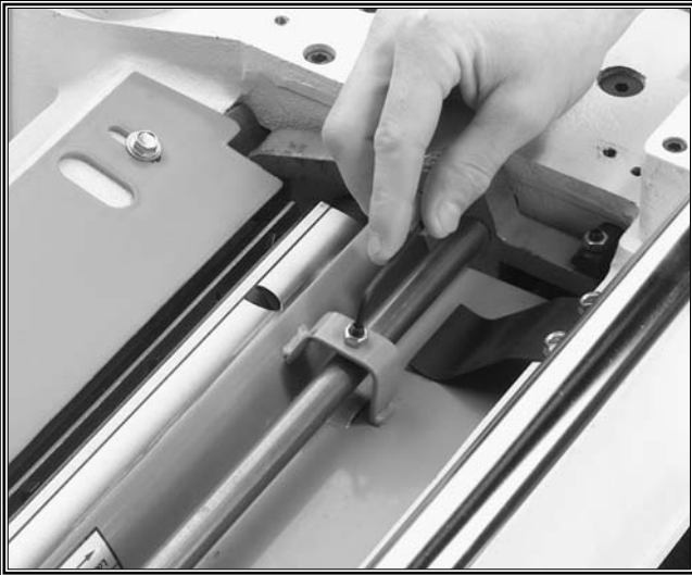
Figure 22. Chipbreaker adjustment controls.
