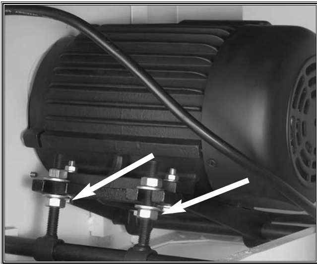
Figure 40. V-belt adjustment check nuts.
