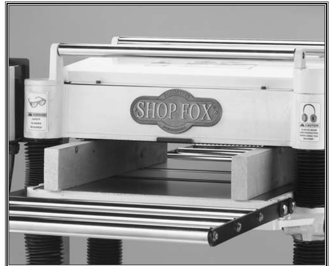
Figure 19. Board position on table.
