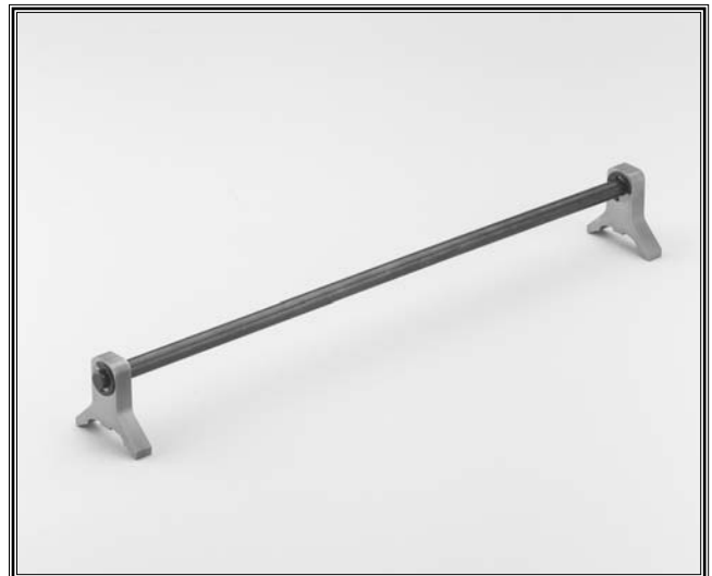
Figure 7. Knife setting jig.
