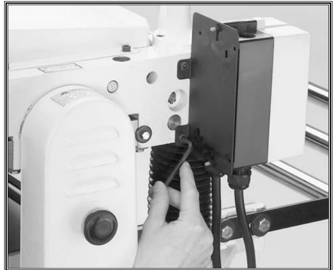
Figure 6. Attaching switch to the planer.
