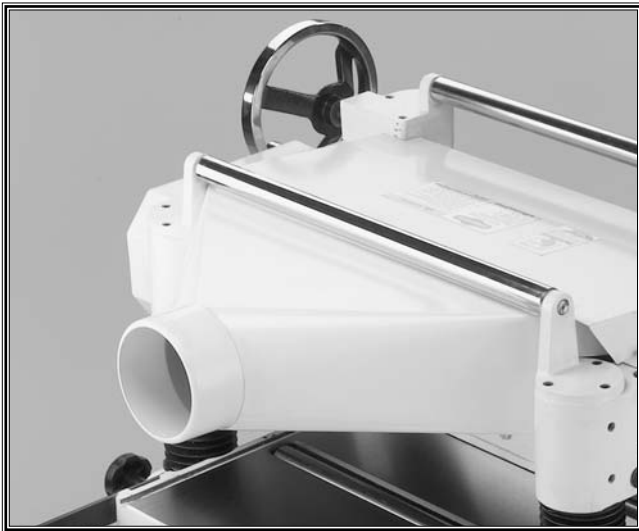
Figure 5. Dust hood attached to planer.
