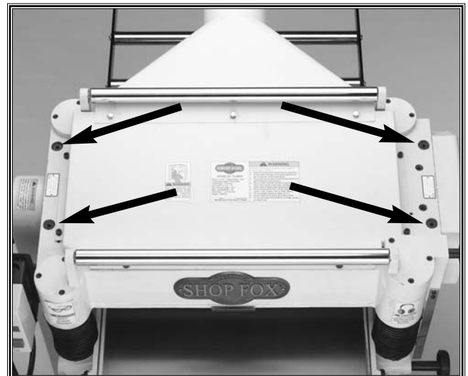
Figure 39. Bearing lubrication points.
