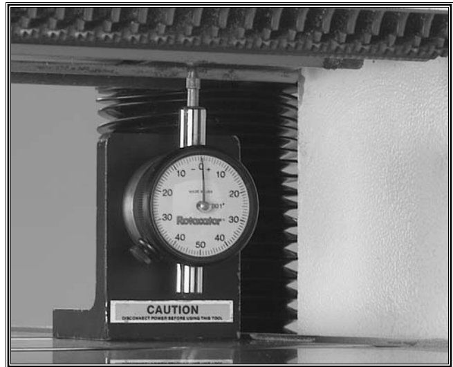
Figure 34. Measuring table-to-cutterhead with Rotacator® in upward position.
