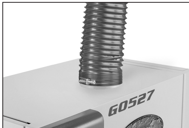
Figure 8. Example of hose attached to port.
