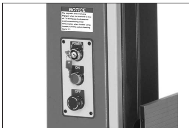
Figure 4. G0531B switch disabling key and ON/OFF buttons.
