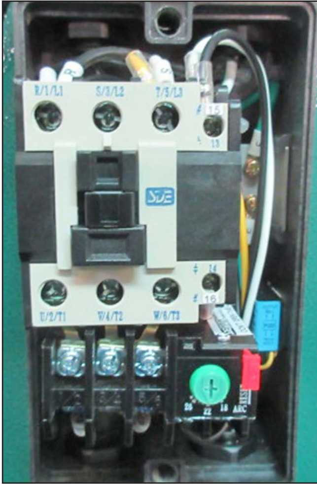
Figure 10. G0531B magnetic switch.
