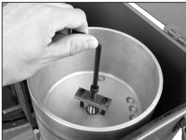
Figure 36. Using the drive roller puller.
