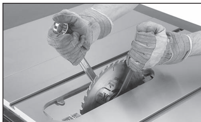
Figure 60. Loosening arbor nut.
