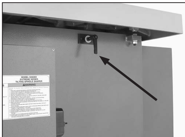
Figure 20. Spindle tilt side lock (right side shown accessed underneath the table).
