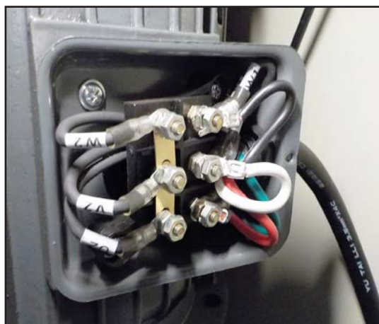
Figure 59. Motor junction box wiring (220V).
