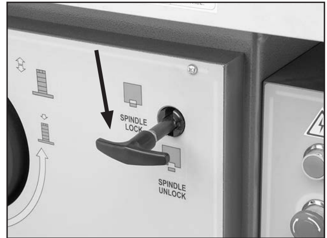
Figure 17. Spindle rotation lock in locking position.
