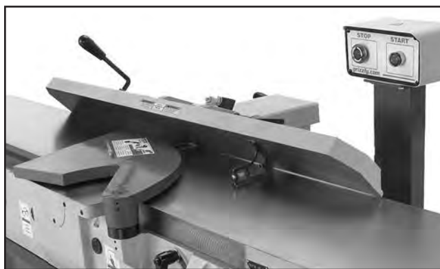
Figure 57. Fence adjusted 45° inward.
