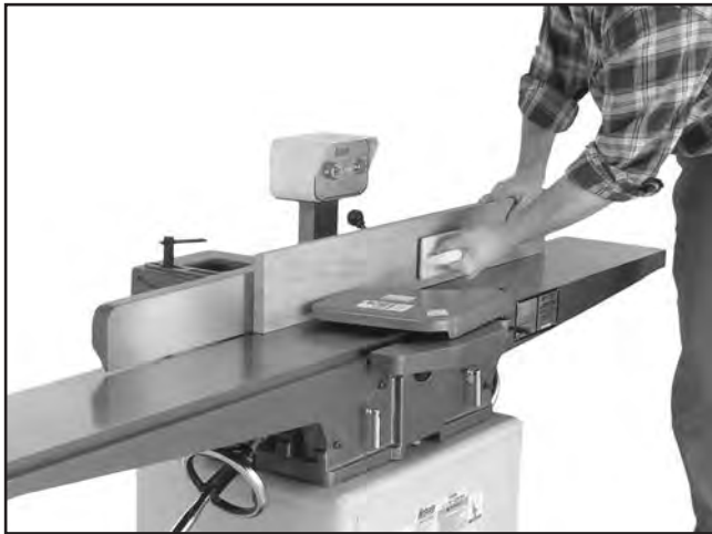
Figure 24. Typical edge jointing operation.
