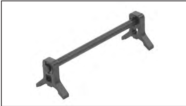
Figure 13. Knife setting jig assembly.
