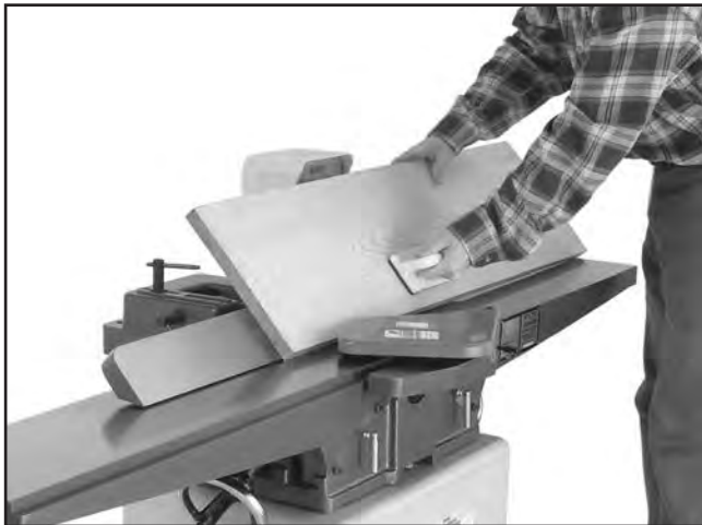
Figure 26. Typical bevel cutting operation.
