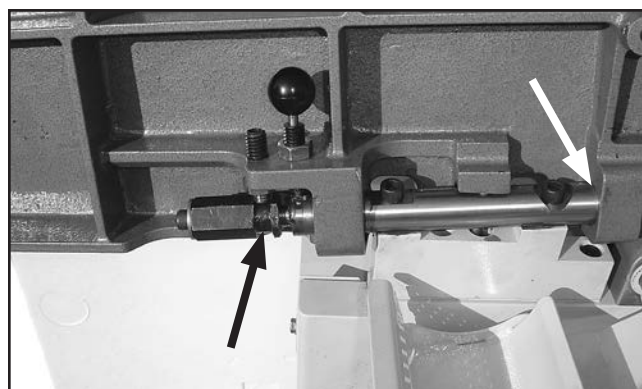
Figure 58. Jointer outfeed table lubrication locations.
