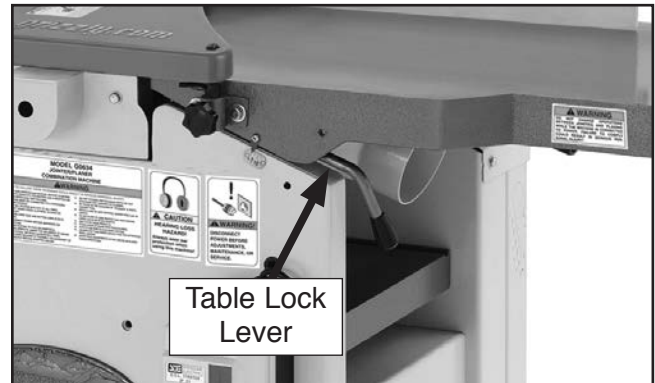
Figure 39. Example of infeed table lock lever.
