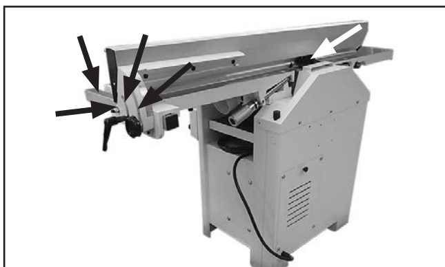
Figure 56. G0634XP fence lubrication locations.
