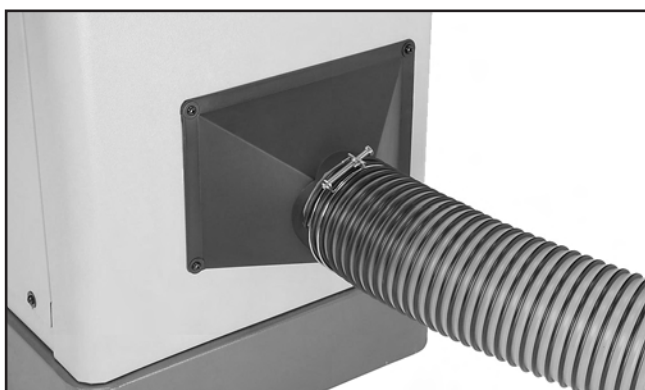
Figure 17. Dust hose attached to dust port.
