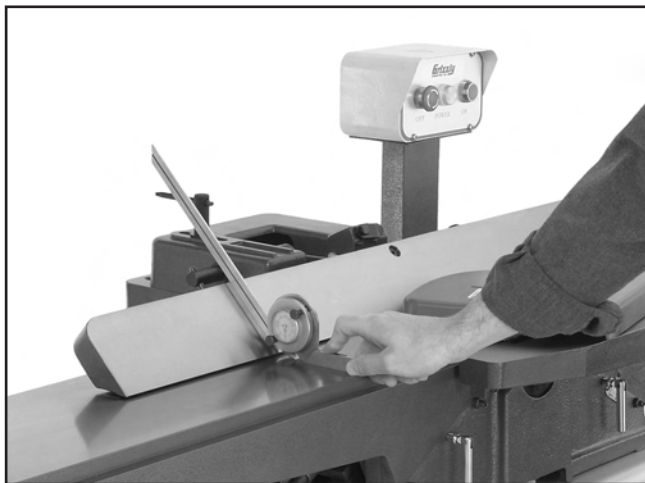
Figure 62. Example of adjusting fence 45° outward.
