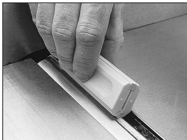
Figure 37. G3631 Jointer/Planer Knife Hone.
