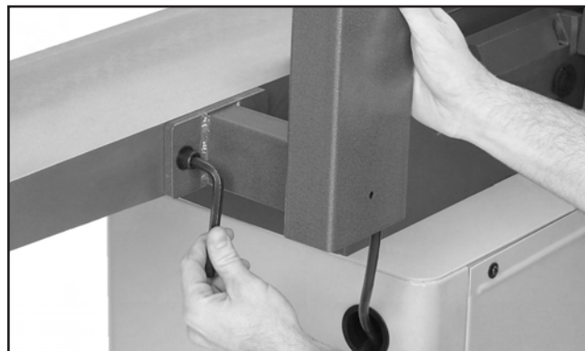
Figure 15. Attaching pedestal switch to stand.
