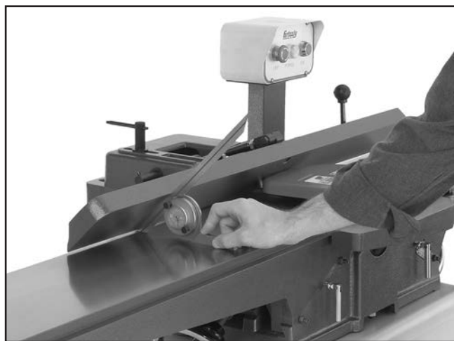
Figure 58. Example of adjusting fence 45° inward.
