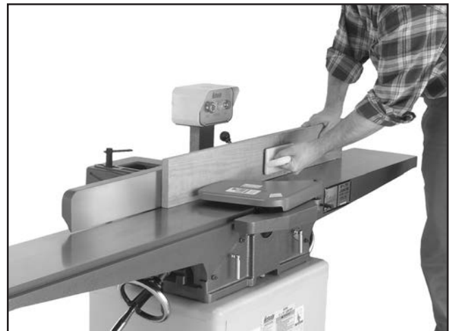
Figure 28. Typical edge jointing operation.
