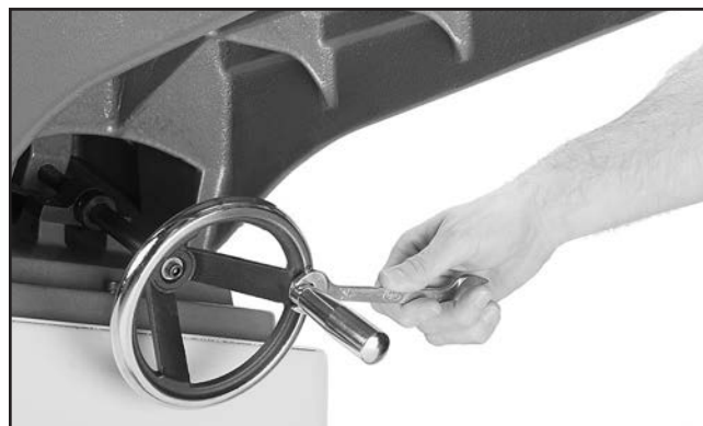
Figure 12. Securing the handwheel handle.
