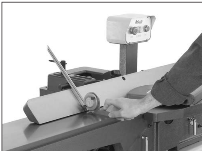
Figure 62. Example of adjusting fence 45° outward.
