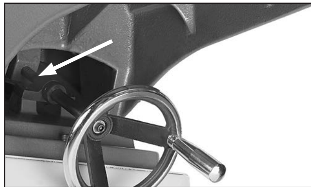
Figure 46. Leadscrew lubrication location.
