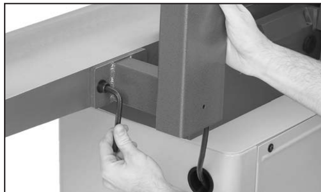
Figure 15. Attaching pedestal switch to stand.
