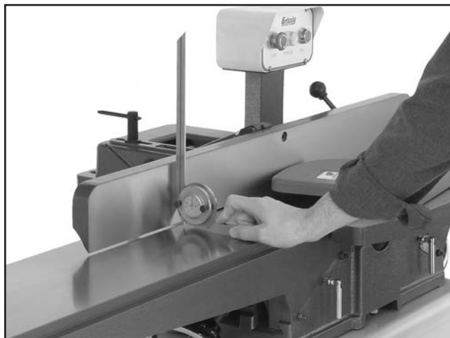
Figure 60. Example of adjusting fence to 90°.
