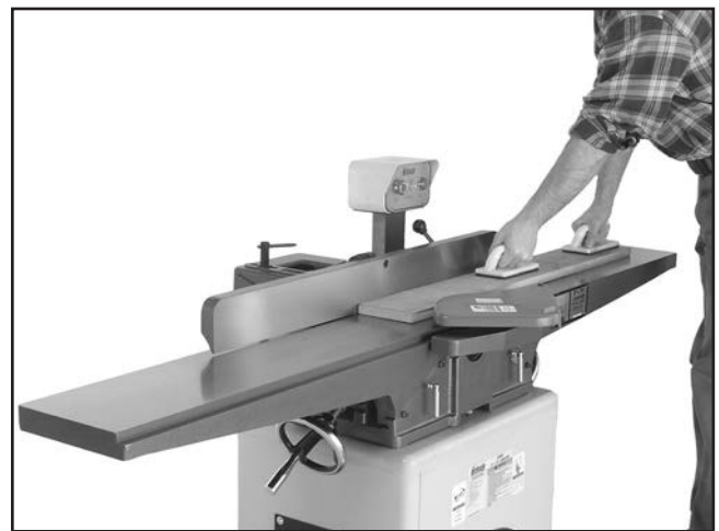
Figure 26. Typical surface planing operation.
