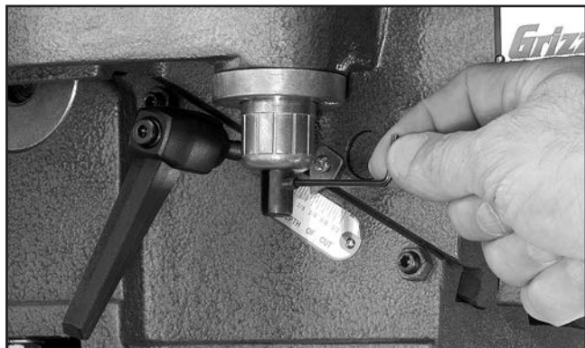
Figure 14. Example of installing cutterhead guard set screw.
