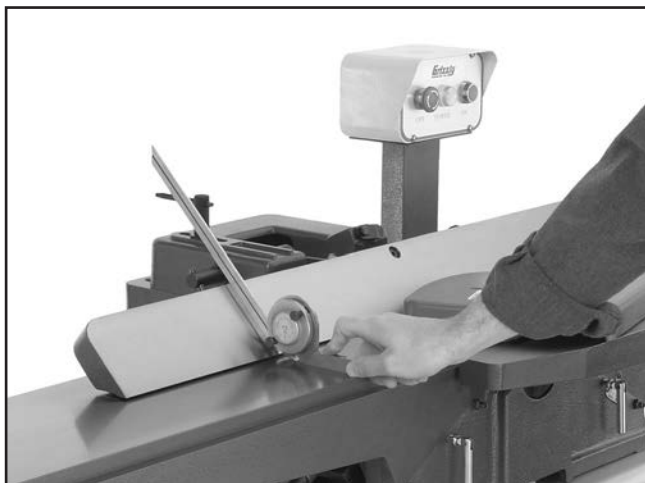
Figure 72. Example of adjusting fence 45° outward.
