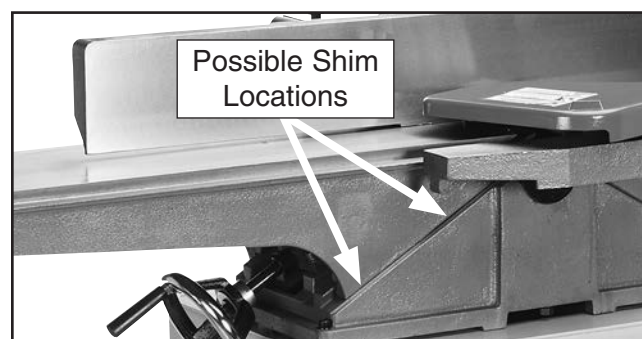
Figure 79. Locations to place shims when adjusting table parallelism.
