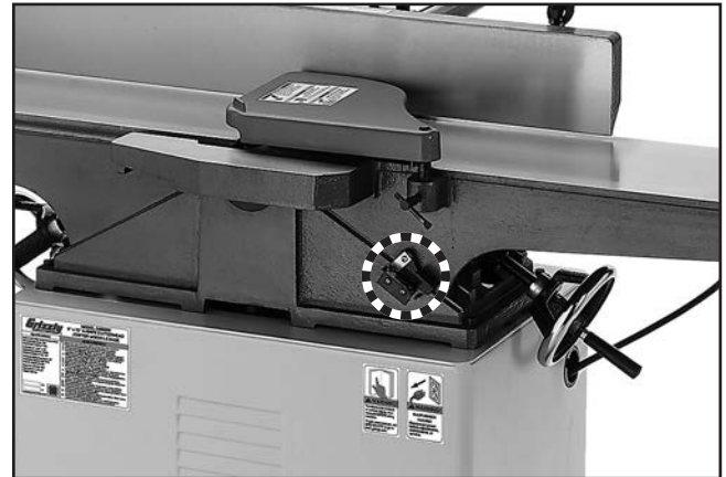
Figure 35. Location of depth-of-cut scale.
