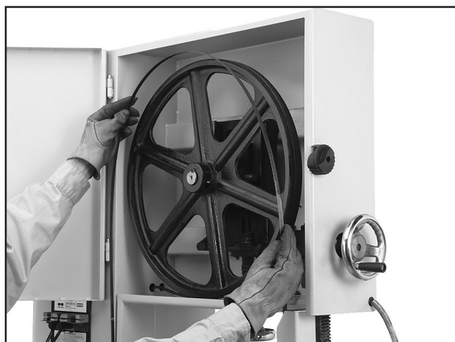
Figure 17. Placing blade on upper wheel.
