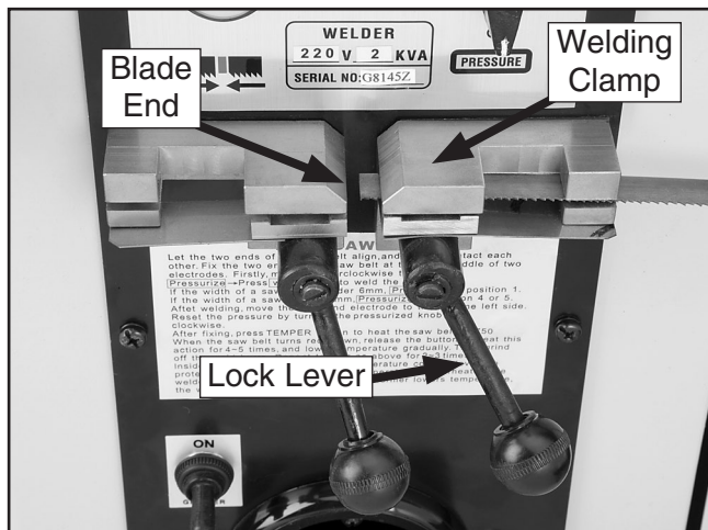
Figure 29. Blade end properly position in welding clamp and locked in place.
