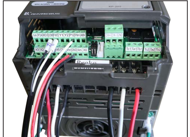
Figure 4. Inverter/Controller box wiring (see wiring diagram on Page 3 ).
