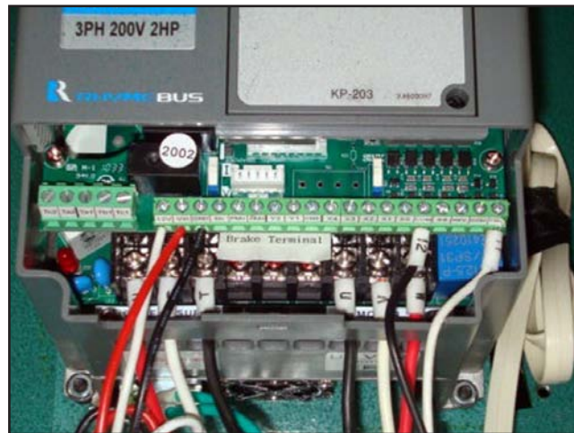
Figure 56. Inverter/Controller box wiring (see wiring diagram on Page 43 ).
