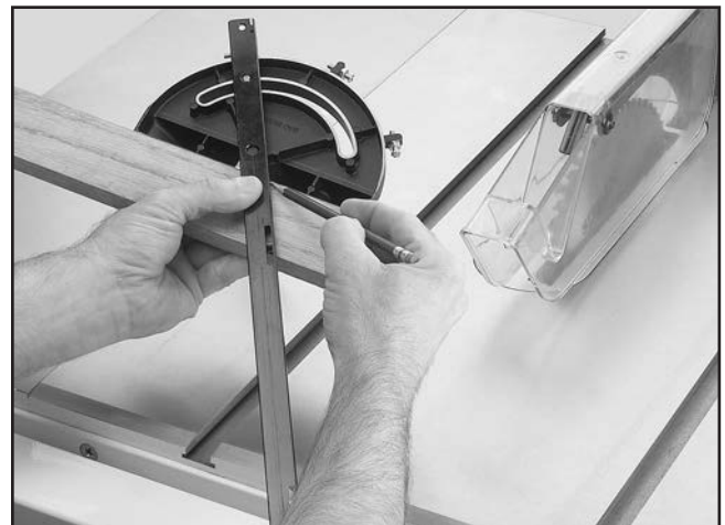
Figure 56. Example of marking miter line.
