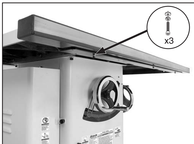
Figure 19. Model G0690 tube attached to front rail.
