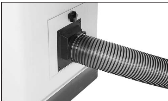
Figure 35. Dust hose attached to dust port.
