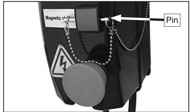
Figure 38. Switch disabling pin inserted into ON button.
