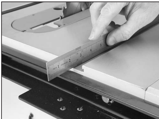
Figure 22. Verifying rear rail is flush with bottom of T-slot.
