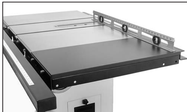
Figure 24. Adjusting Model G0690 extension table flush with extension wing and table.
