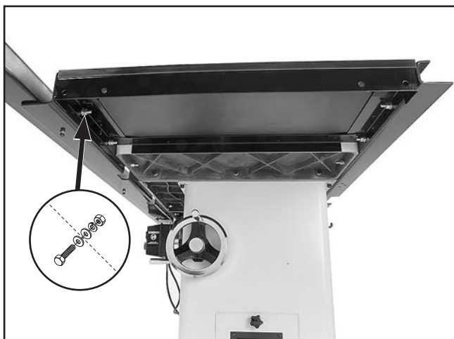
Figure 23. Model G0690 extension table installed.
