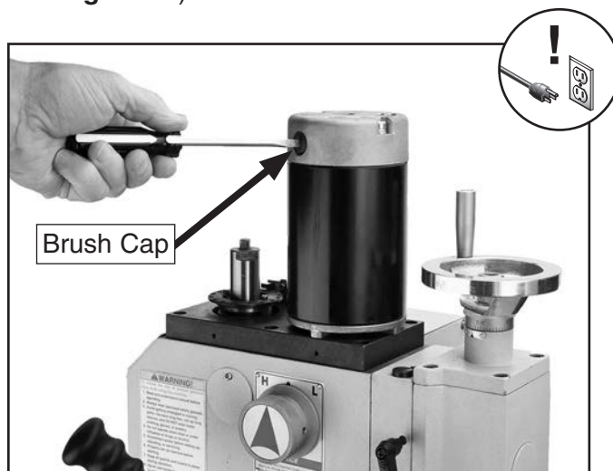
Figure 47. Removing motor brush cap.
