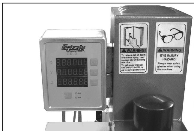
Figure 1. DRO magnetically mounted to mill headstock.
