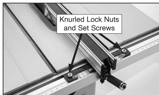
Figure 116. Location of lock nuts and set screws for adjusting fence squareness and height.
