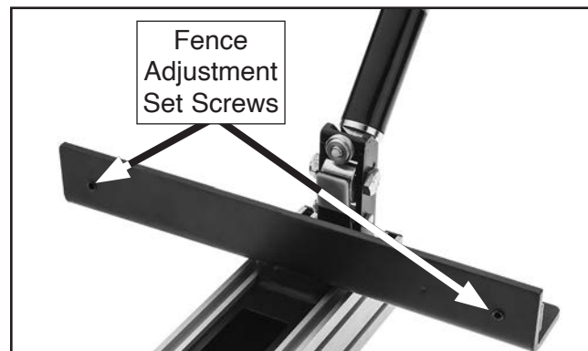
Figure 123. Location of set screws to adjust fence parallelism (shown upside down).
