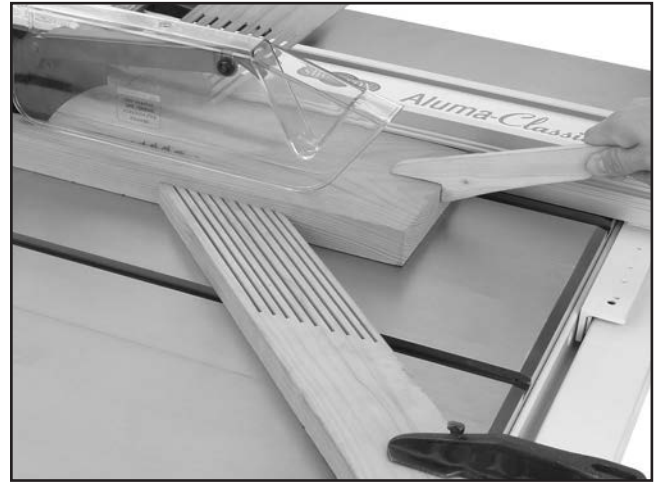
Figure 53. Typical ripping operation.
