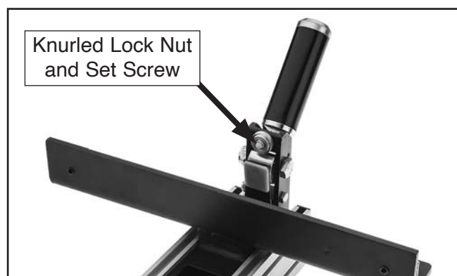
Figure 122. Set screw for adjusting fence handle clamping pressure.
