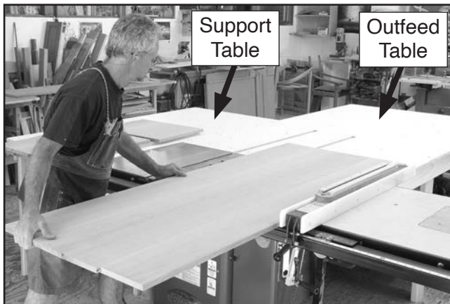
Figure 90. Example of outfeed & support tables.
