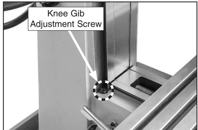
**Figure 72.** Knee gib adjustment screw (1 of 2).
