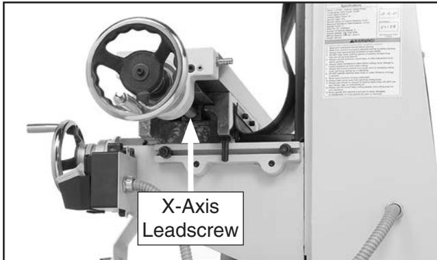
**Figure 58.** X-axis leadscrew as viewed from the underneath right side of the table.
