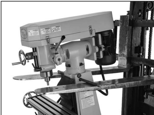
**Figure 15.** Lifting Model G0801/G0802.
