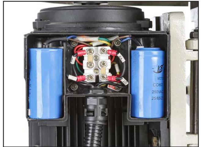
Figure 84. 110V motor wiring.
