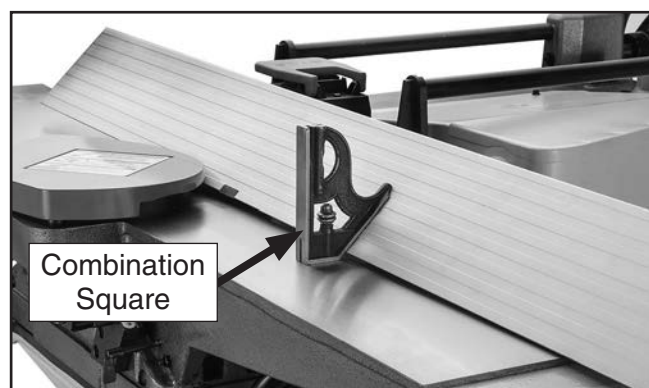
Figure 74. Fence adjusted to 135° (45° outward).
