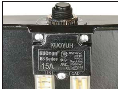
Figure 100. Main motor circuit breaker wiring.
