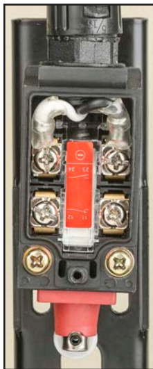
Figure 105. Saw Down limit switch wiring.
