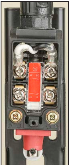
Figure 105. Saw Down limit switch wiring.
