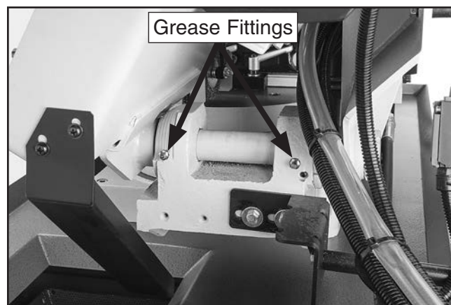
Figure 69. Pivot-point grease fitting locations.
