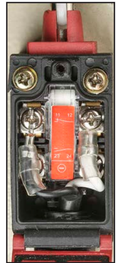
Figure 107. Blade cover limit switch wiring.
