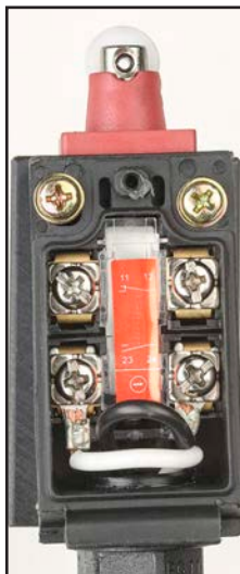
Figure 106. Saw Up limit switch wiring.
