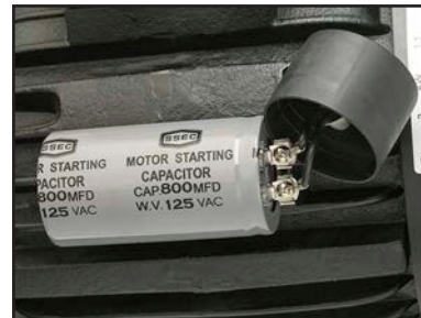
Figure 102. Main motor start capacitor wiring.
