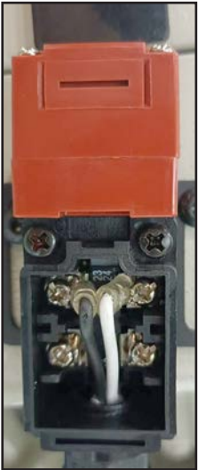
Figure 107. Blade cover limit switch wiring.
