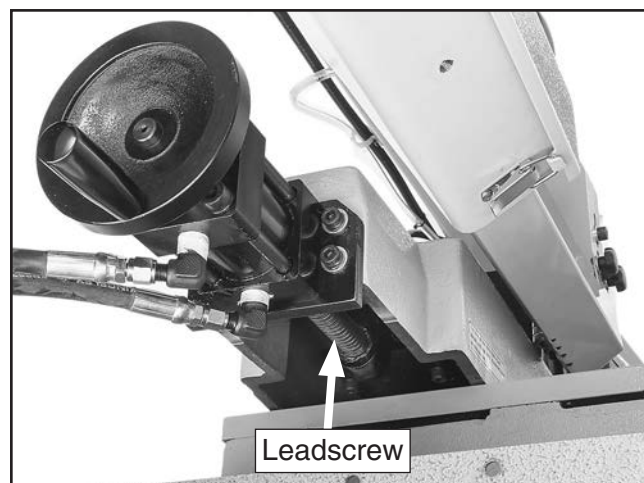
Figure 66. Vise leadscrew lubrication area.
