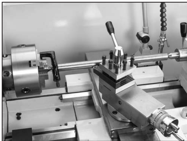
Figure 46. Example photo of stock mounted between the centers.
