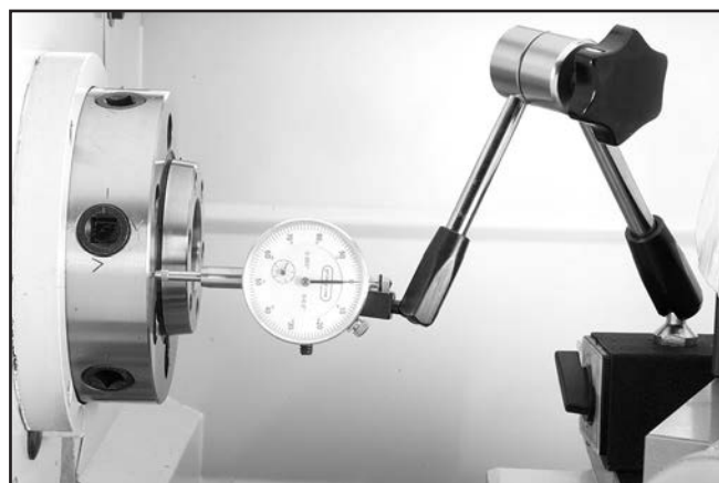
Figure 139. Example of dial indicator setup.
