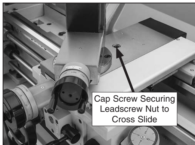
Figure 120. Location of cap screw that secures the leadscrew nut.
