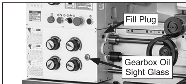
Figure 105. Location of gearbox oil sight glass and fill plug.
