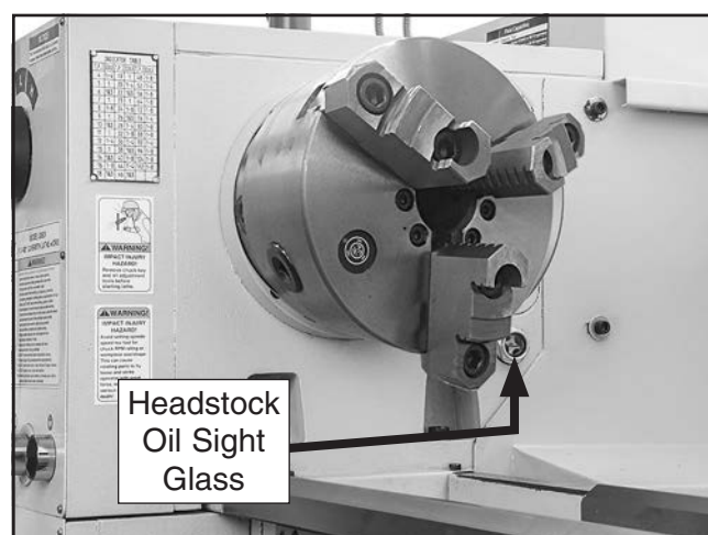
Figure 103. Location of headstock oil sight glass.
