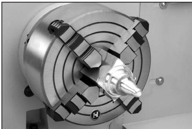
Figure 38. Example of non-cylindrical workpiece correctly mounted on the 4-jaw chuck.
