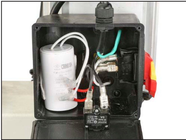
Figure 41. Motor junction box components.
