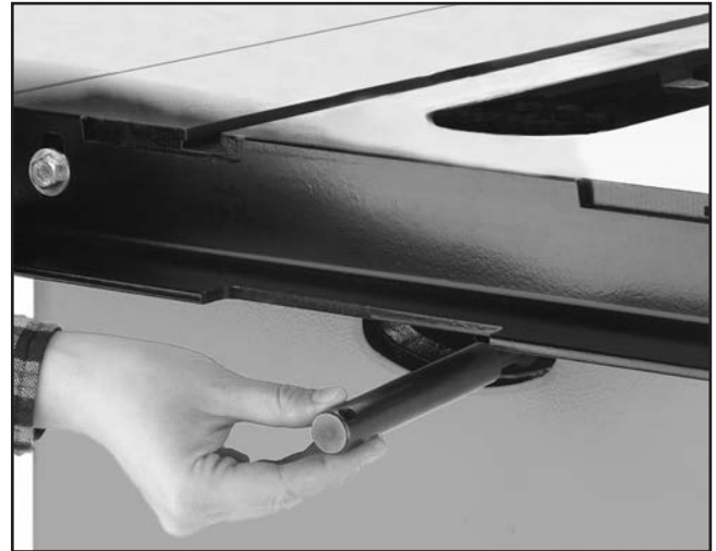
Figure 12. Attaching guard support shaft.
