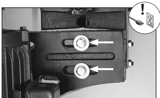
Figure 70. Location of motor mount hex bolts.
