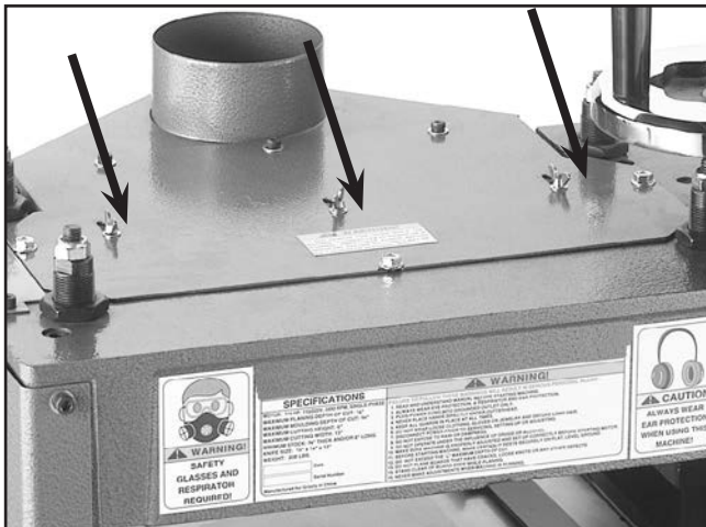
Figure 14. Dust hood installed.
