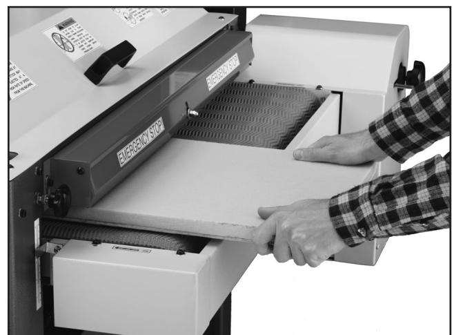
Figure 35. Example of using D3003 PRO-STIK® Cleaning Pad to clean sandpaper.
