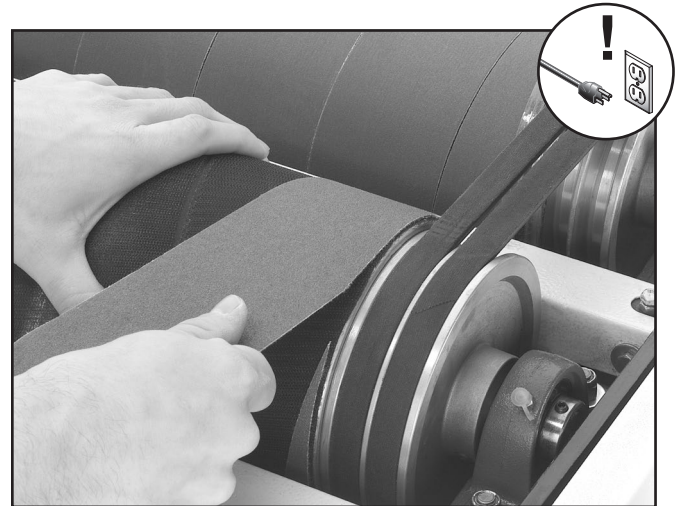
Figure 27. Example of wrapping sandpaper around drum.
