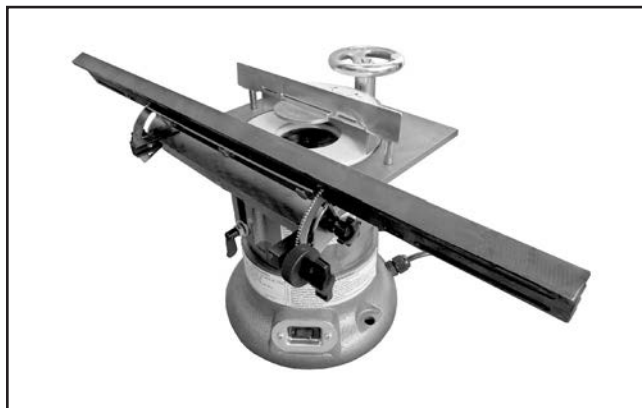
Figure 18. Pivot support and slide table assembly properly attached to table.
