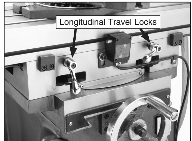
Figure 30. Longitudinal feed lock locations.
