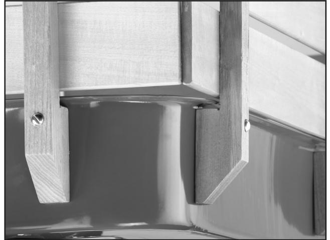
**Figure 3.** Wood stake side mounted to the outside of the bed.
