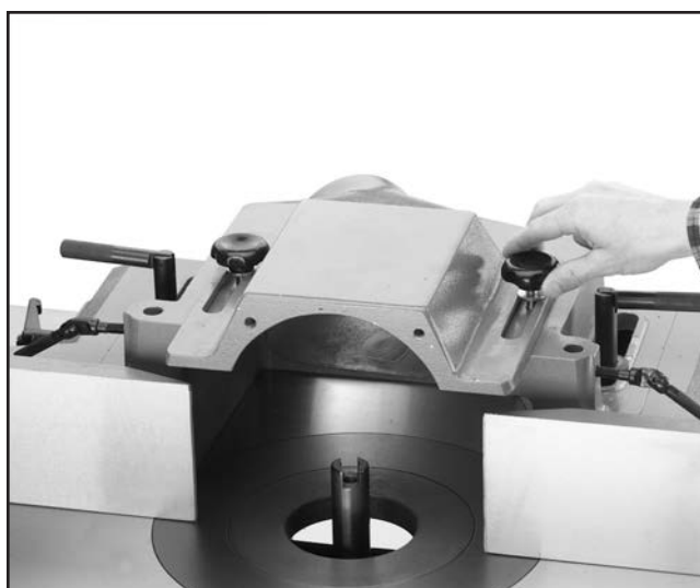
Figure 6. Installing the cutter guard.
