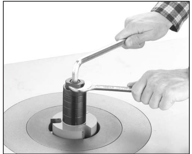
Figure 15. Tightening spindle nuts.
