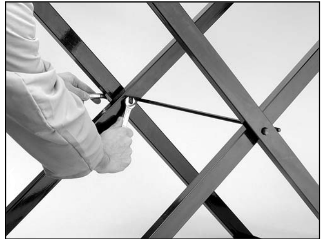
Figure 4. Assembling the stand brackets.
