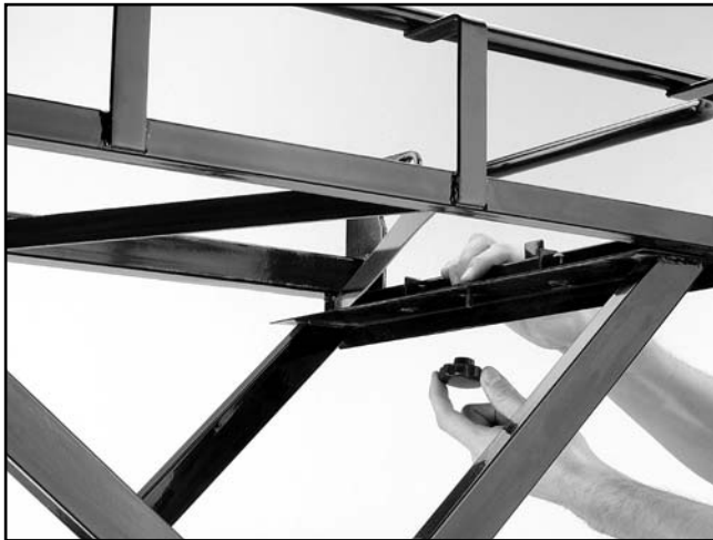
Figure 6. Mounting the saw frame to the stand.
