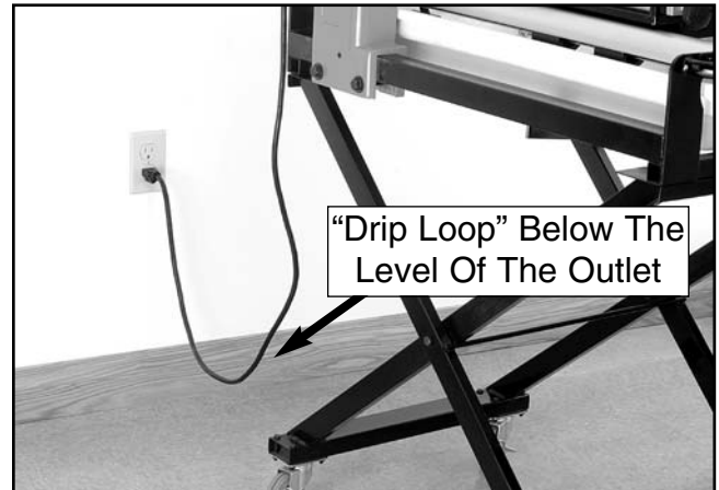
Figure 18. Correct cord positioning.
