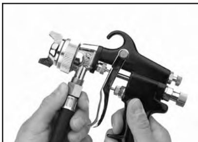
Figure 4. Attaching fluid hose to spray gun.
