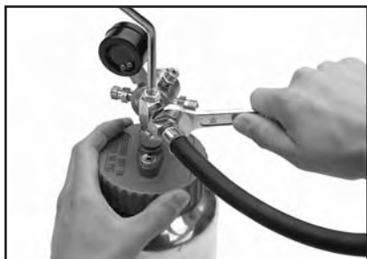
Figure 3. Installing fluid hose.
