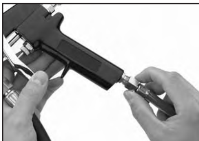
Figure 6. Attaching hose to spray gun.
