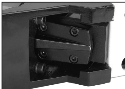
Figure 6. Cap screws securing the magazine.
