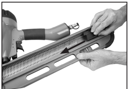
Figure 5. Releasing the pusher.
