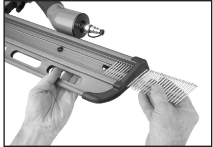
Figure 3. Loading nails in the magazine.
