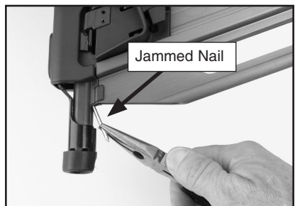
Figure 11. Using pliers to remove a jammed nail.
