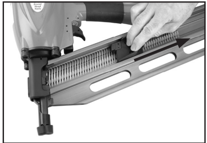
Figure 4. Pulling the pusher back.
