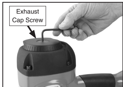
Figure 8. Loosening the exhaust cap screw.
