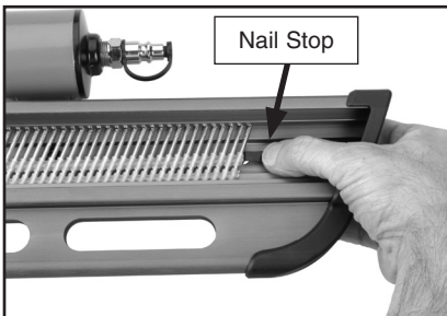
Figure 7. Pressing the nail stop down.
