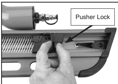
Figure 6. Pulling the pusher back and releasing the pusher lock.
