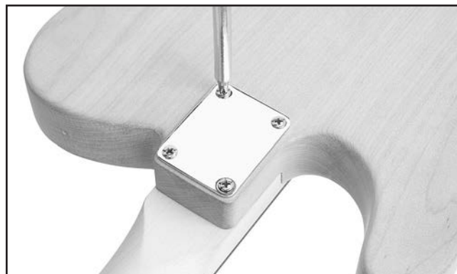
Figure 12. Fastening neck to body.
