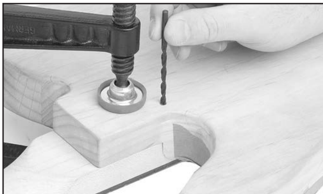
Figure 10. Making a pilot hole in the neck.
