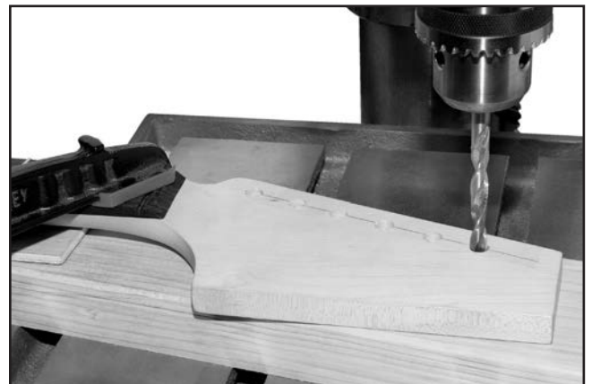
Figure 7. Drilling the pegholes.
