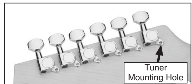
Figure 21. Tuners aligned to edge of headstock.
