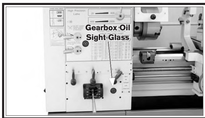
Figure 112. Gearbox sight glass location.
