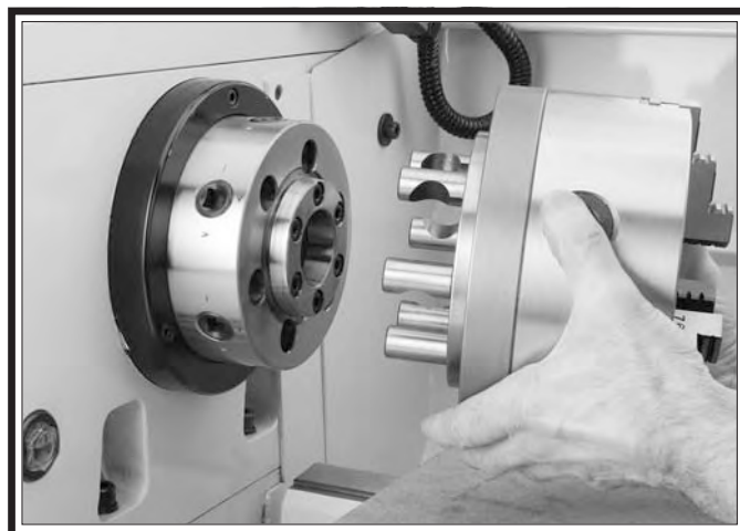
Figure 41. Example of removing a 3-jaw chuck from a spindle nose.
