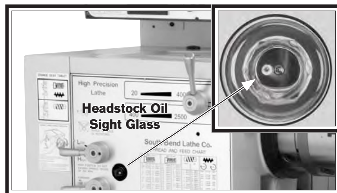
Figure 109. Location of the headstock oil sight glass.
