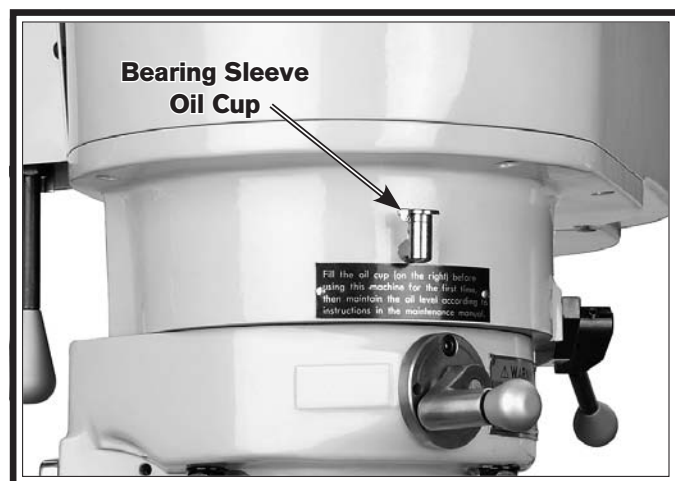
Figure 48. Speed range bearing sleeve.
