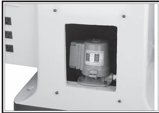
Figure 57. Location of coolant pump.
