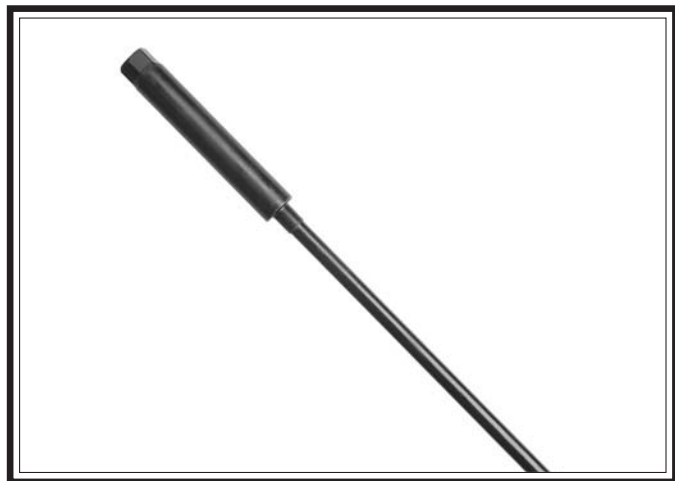
Figure 43. Spindle drawbar and spacer.
