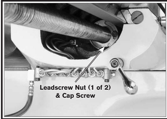
Figure 61. Longitudinal leadscrew nut and cap screw, as viewed from underneath the left side of the table.
