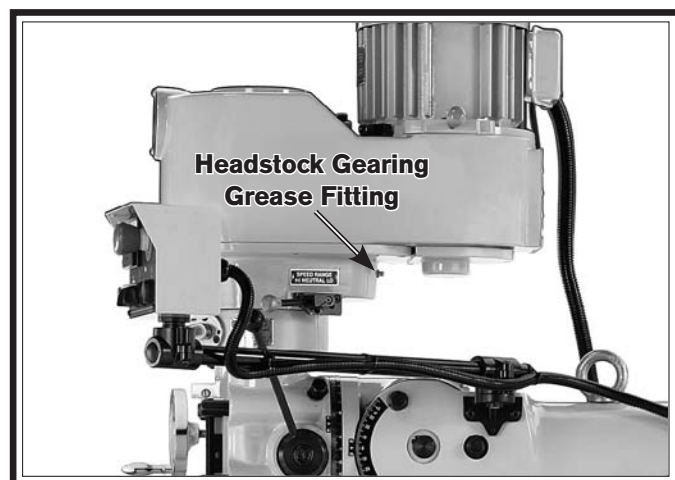
Figure 49. Headstock gearing grease fitting.
