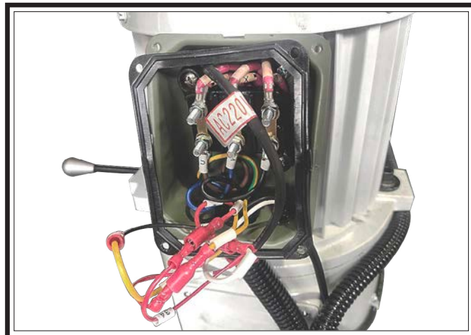
Figure 68. Spindle motor wiring.
