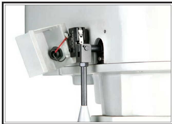
Figure 69. Spindle brake switch wiring.
