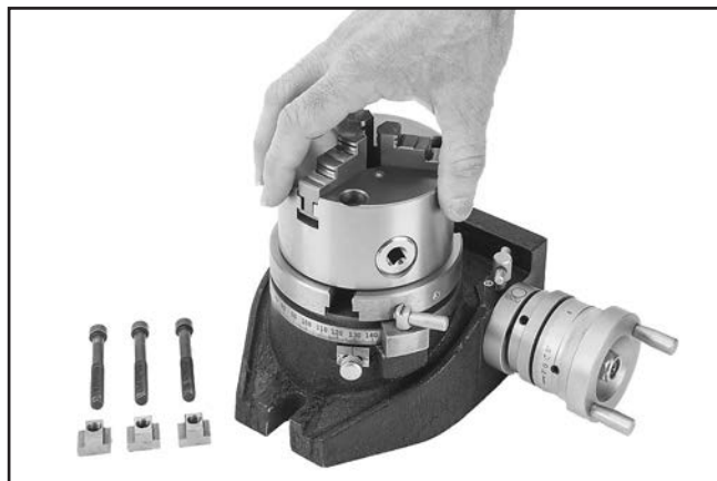
Figure 15. Mounting chuck to rotary table.
