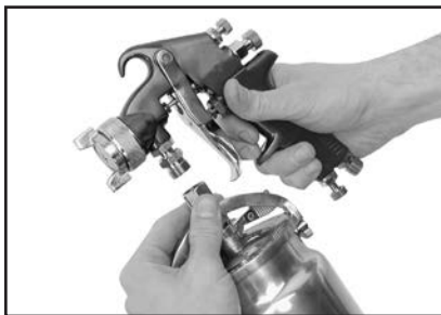
Figure 3. Example of attaching spray gun body to fluid cup.
