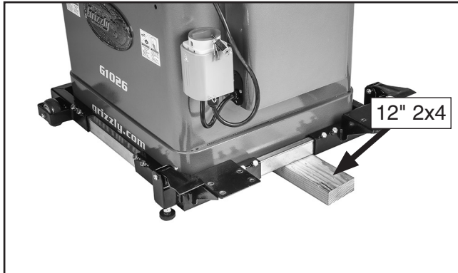
Figure 20. 2x4 Placed beneath machine and mobile base frame.
