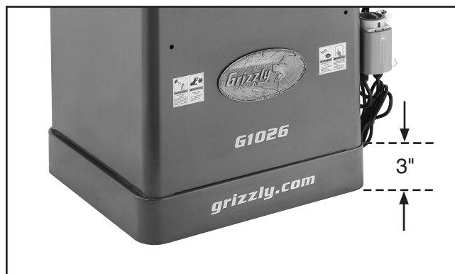
Figure 3. Example of 3" high band around machine base.
